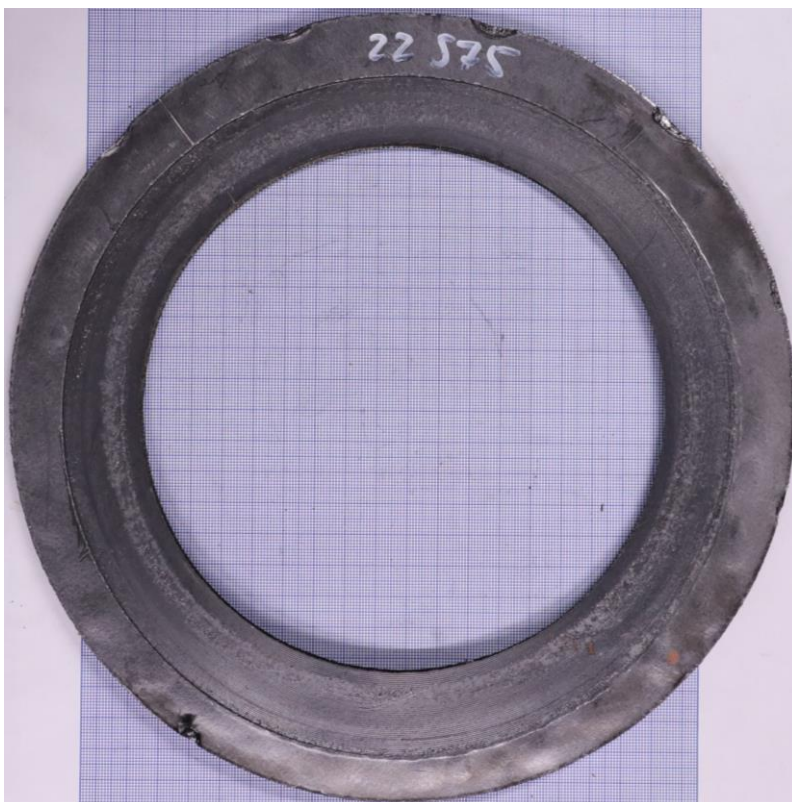
SIGRAFLEX iNXT V20010C5N after Fire Test 22-575 according to API Specification 6FB
