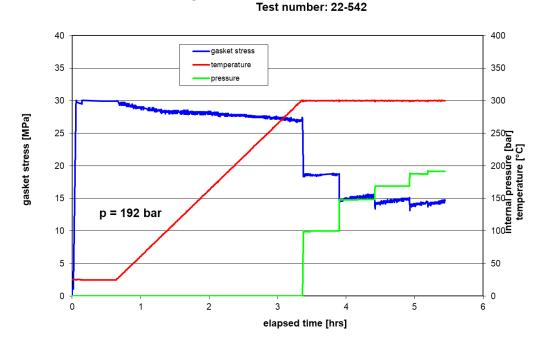
Hot Blow-Out Test HOBT Sigraflex iNXT V20010C5N 136.85x89.1x2.08 mm Test number: 22-542
